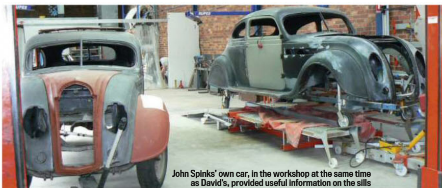
Templates from another Airflow were used to fabricate new sills
