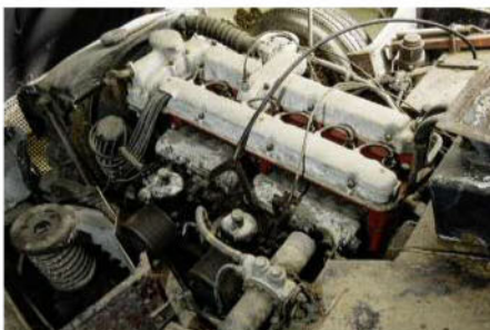
Suspension turrets need replacing. And that's just for starters
